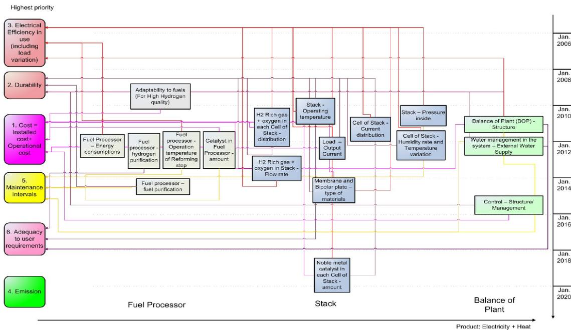
Figure 18. Map of contradiction for low temperature small fuel cell technologies with time scale. Source: [33] (Information provided courtesy of EIFER, 2005, Karlsruhe)
